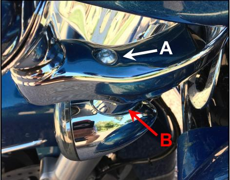
Water is entering the turn signal housing from one of two places. Water can enter through the Allen head mounting bolt (See Arrow A). Water can also enter through the top and bottom of the turn signal mount (See Arrow B).
