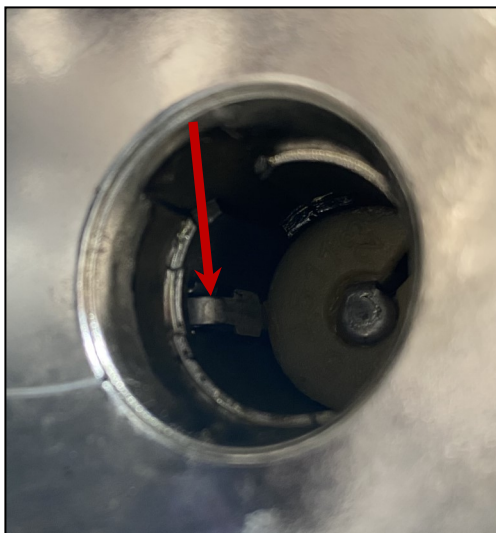
Check that the ground connection tab is properly raised from the socket and in place.
