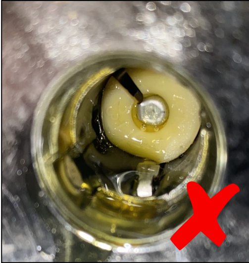
An example of a 1156 socket with dielectric grease.
